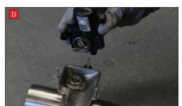
be able to see the torsion spring (This must stay on the electronic valve motor to work with Scorpion Exhaust).
